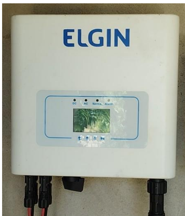
Figura 16 – Inversor solar On-grid
